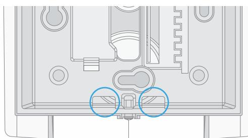
On the top of the mounting plate, there is also two pilot holes (shown below) for possible cable entries. Please use a drill (max. diameter of 6mm) to make the hole. When using a drill, ensure that the base plate is firmly clamped. Before drilling, the pressure must be reduced - sudden break-through of the drill bit can be the result.
